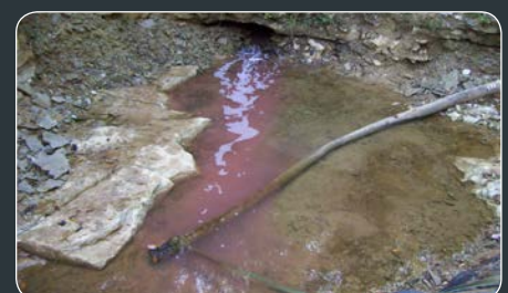
RHODAMINE WT (RED) DYE TRACER TESTING AT SPRING 018
